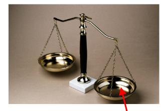
To measure the mass of an object, the object is placed on one pan and **standard masses** are placed on the other pan until the pans *balance* each other. The mass of the object is the sum of the standard masses on the other pan.
